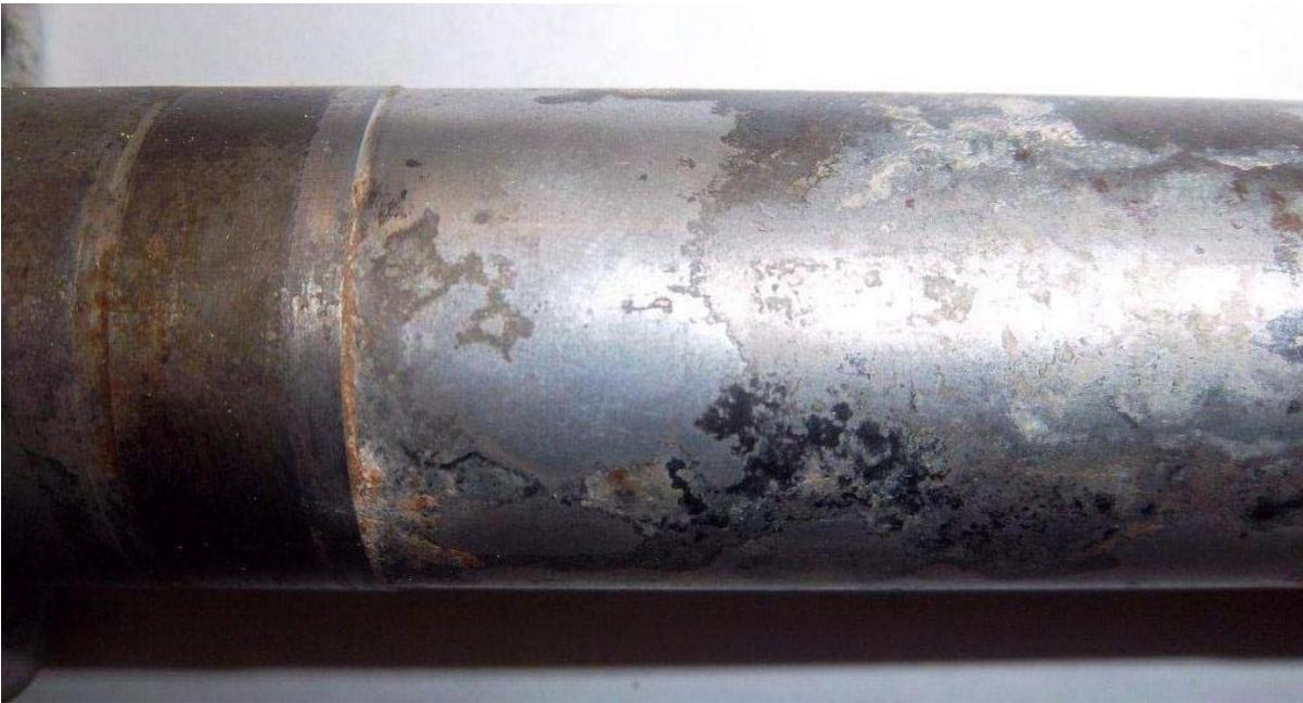
**De Havilland DHC8103, Corroded Aileron Control Shaft, ATA 2710**
